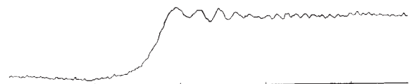
Fig. 1. Facsimile of observed occultation curve at 430 Mc/s using 1-Mc/s bandwidth and smoothed with a time constant of 1 sec. Horizontal scale: universal time, 1 div. represents 1 min
