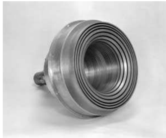
Figure 3 The CSIRO-designed Apollo feed horn (Photo: CSIRO).
